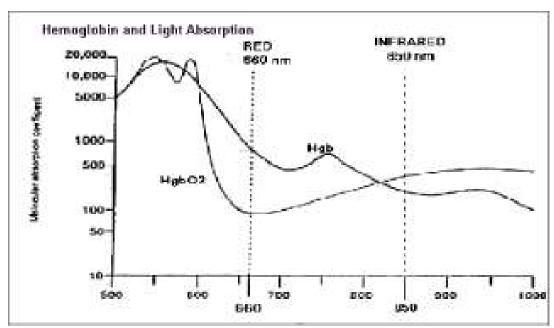
Figure 2 Red light attenuation in oxygen rich and oxygen starved hemoglobin (Elwell 1999)
